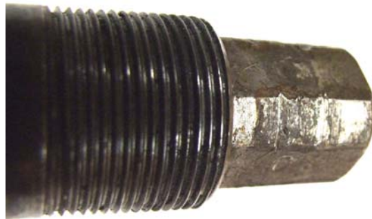
loupe crosses joint connection (the corrosion of that axle)
